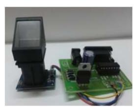
R305 Fingerprint Module is a serial unique finger impression scanner which can be straightforwardly associated with the PC's comport. R305 Fingerprint Sensor can undoubtedly be associated with any controller by means of MAX232 IC. This Fingerprint scanner is fit for putting away and looking at the unique mark and as needs be giving the wanted yield.
